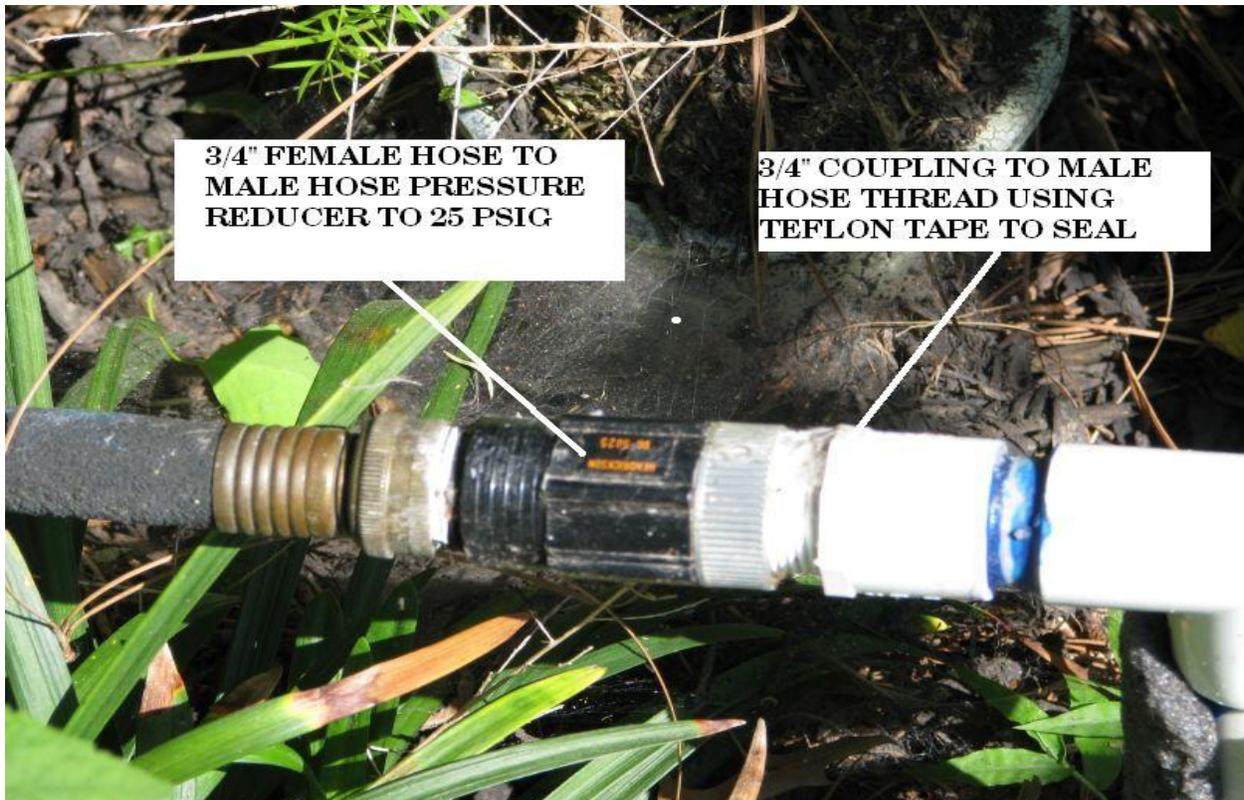
An existing 3/4" riser for a pop up 1.5 GPM sprinkler head has been modified by adding a tee, 3/4" coupling with hose threads. A pressure reducer fitting is screwed on the 3/4" hose thread side of coupling and soaker hose is connected to the pressure reducer. Teflon tape is used to seal threaded connections.
